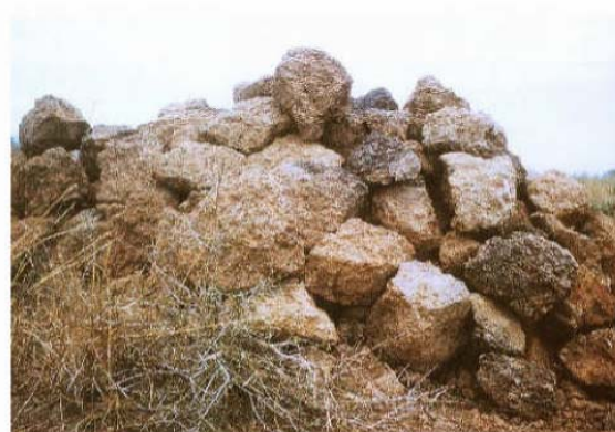
Photo 2-6: Stockpiled hardpan laterite boulders
